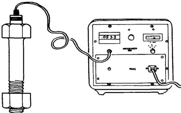
**Fig. 35.29** An acoustic transducer is held against one end of the fastener to measure the fastener's change in length as it is tightened.
