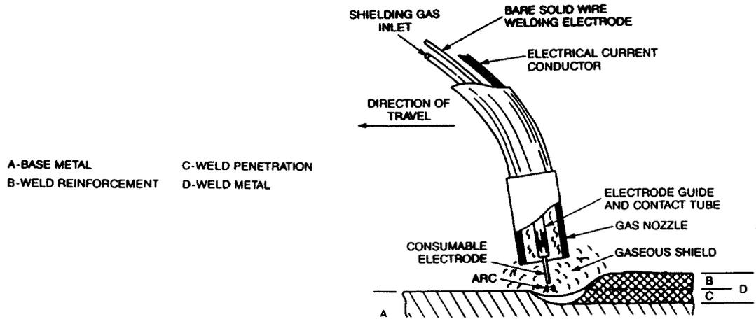
Fig. 35.34 Diagrammatic sketch of (GMA) welding process.
