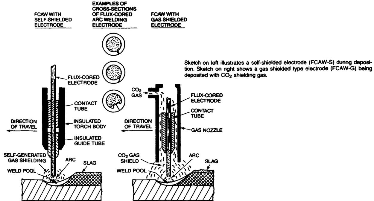
**Fig. 35.36** Diagrammatic sketches of the flux-cored arc welding process.
