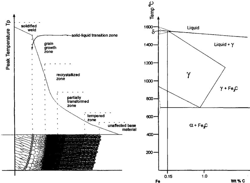
**Fig. 35.39** A schematic of the various subzones of the HAZ for the alloy indicated on the Fe-Fe<sub>3</sub>C equilibrium diagram.
