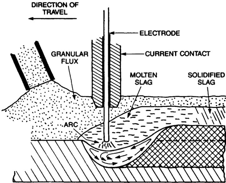
**Fig. 35.31** Diagrammatic sketch of the submerged arc welding process (SAW). Sketch illustrates electrode deposition on a thick plate, Arrows drawn on weld pool show the usual hydrodynamic motion of the molten metal.
