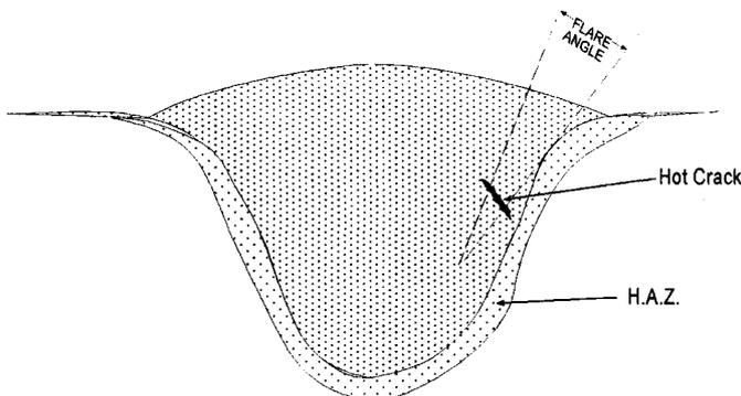
**Fig. 35.33** Weld made by SAW with flare angle and hot cracking at juncture of 2 solidification fronts.
