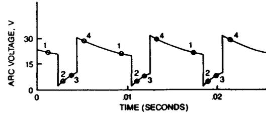
Fig. 35.35 GMAW process operating in the short-circuiting transfer mode.
