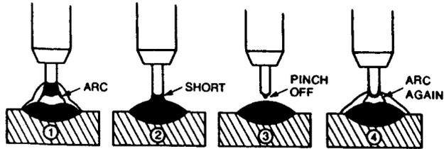
THE SHORT CIRCUITING TRANSFER MECHANISM ILLUSTRATED ABOVE MAY BE REPEATED CYCLICALLY AT A FREQUENCY RANGING FROM ABOUT 20 TO MORE THAN 200 TIMES/SECOND.
