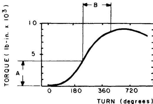
**Fig. 35.28** In turn-of-nut techniques, the nut is first tightened with an approximate torque (A) and then further tightened with a measured turn (B).
