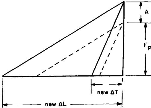
**Fig. 35.27** The external load applied to the joint interface has exceeded the critical load by an amount = *A*.
