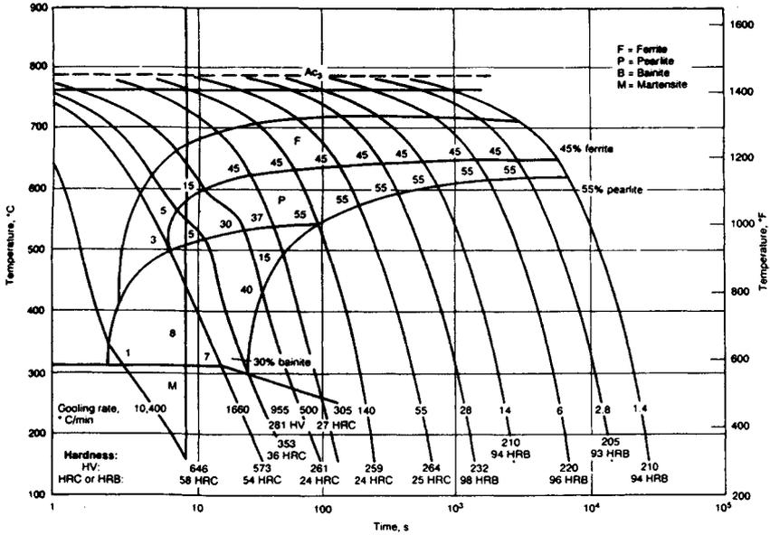
**Fig. 35.38** Conventional CCT diagram for an AISI 1541 (.39 C), ASTM grain size 6, austenitized at 980°C. For each of the cooling curves the transformation start and end temperature are given as well as the hardness.
