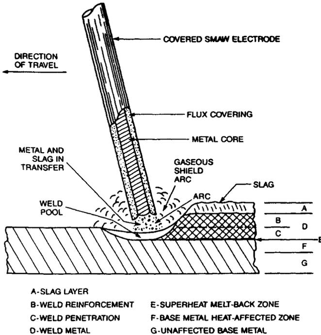
**Fig. 35.37** Diagrammatic sketch of the shielded metal arc welding process (SMAW) using a consumable flux-covered electrode.
