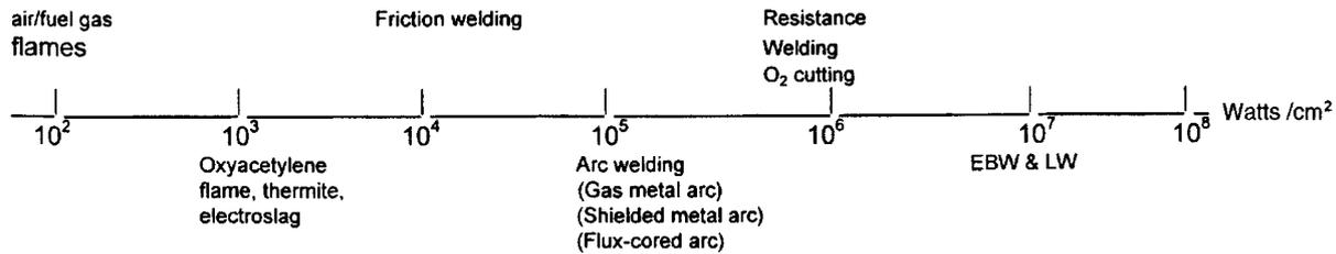
**Fig. 35.30** Spectrum of practical heat intensities used for fusion welding.
