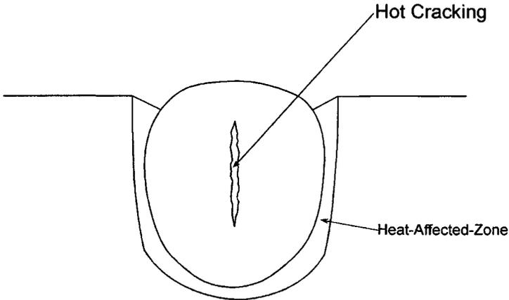
**Fig. 35.32** Deeply penetrating weld made by SAW process with hot cracking.
